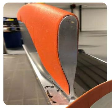
VeeloHEAT Next Generation De-Icing system provides advanced de-ice and antiice protection for next generation composite air vehicles.
